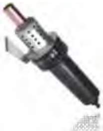
Figure 3 An electric hot-iron dehorner will destroy the horn-producing skin at the base of the horn bud
